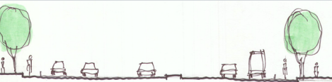
Cross-section of curbside bike lanes on Greenbelt Road. Image Source: ULI Washington.
