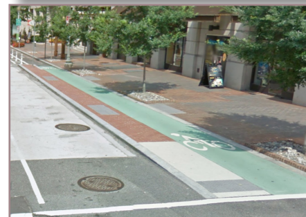
Potential floating bus stop configurations for future consideration. In each, the bike lane briefly raises up to sidewalk level to allow access to the bus boarding area.
